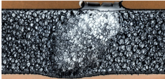
Figure 2. Foam core sandwich panel damage following impact of an aluminum sphere at hypervelocity.
