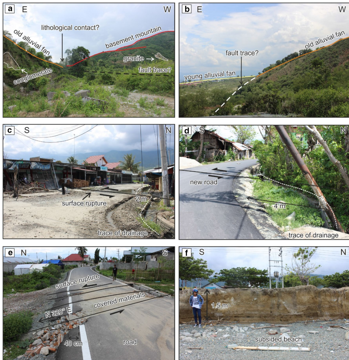
Fig. 3 a A view from STD3-11 showing contact between granite in mountain and conglomerate further east. A depression in between is interpreted as a basin-bounding fault. b A view from STD3-10A showing the relationship between old and young alluvial fan units. A topographic break may indicate a normal fault. c, d Major surface rupture with left-lateral displacement close to Balaroa at STD3-08B and STD3-9B, respectively. e Minor surface rupture at STD3-10B showing left-lateral displacement. f Subsided surface on the beach at STD3-14
