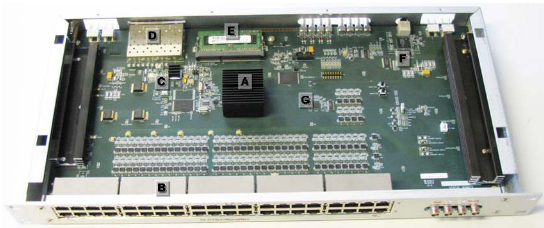
Figure 6. The Scalable Readout Unit (SRU) board: A — Xilinx Virtex 6 FPGA; B — front panel with 40 DTCC connectors (RJ45); C — 10 Gbps Ethernet Phy chip; D — quad SFP+ connector assembly (one 10 GbE and 3 lower speed (< 5 Gbps)); E — DDR3 SO-DIMM socket; F — TTCrx chip; G — jitter-cleaner PLL.
