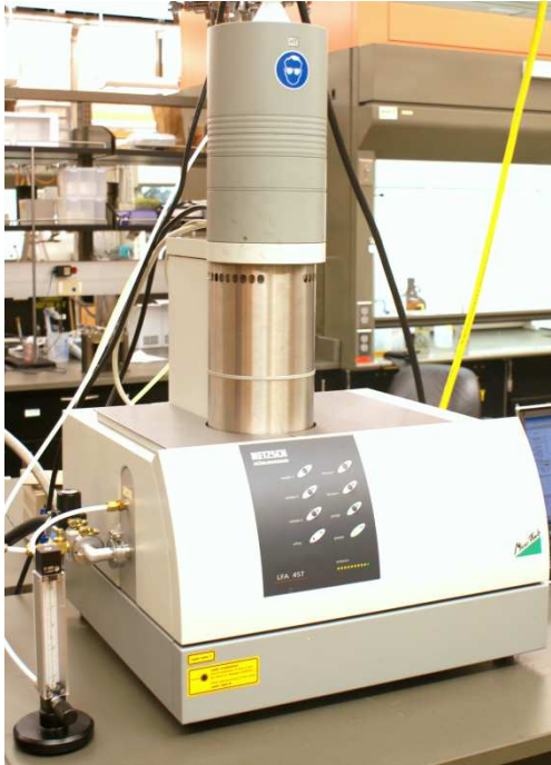
Figure 13: Picture of Netzsch laser flash used for thermal conductivity measurements
