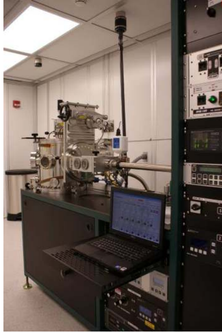
Figure 18 : AJA Orion Sputtering Equipment used for thin film depositions
