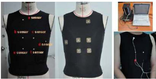
Fig. 3. Developed experimental clothing to measure ECG data and ECG instrument.
