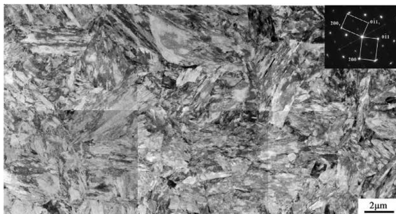
Fig. 1. Microstructure of the oil quenched Fe-0.2C-5Mn after austenization at 750°C with 30 minutes.
