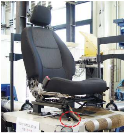
Fig. 7 The position to check exciting modified vibration signal
