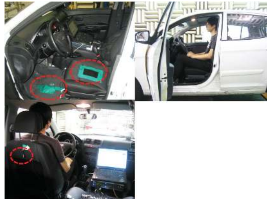
Fig. 4 Photo illustration for the sensor location and driver position for the vibration measurement
