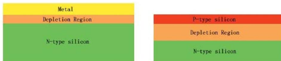
Figure 2.6 Doping profile of Schottky diode (left) and p-n junction diode (right).
