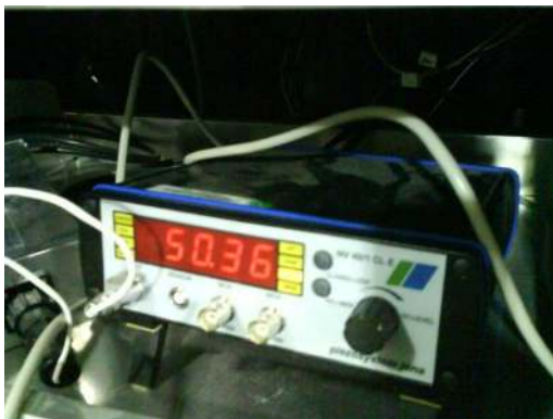
Figure 3.2 Controller for piezoelectric actuator on monochromator at beamline X14A.
