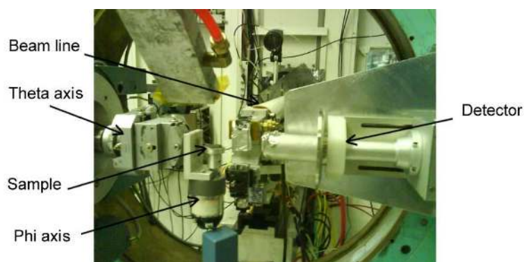
Figure 3.12 Set up of detector without crystal analyzer.
