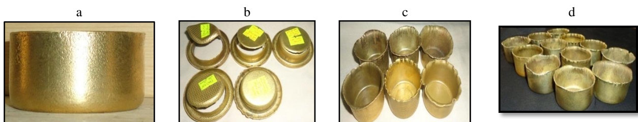
Fig. 7: Samples of Drawen Cups A) Completed Successful Cup, (B,C &D) Cups Produced with Die of Con Angle 45°,15° and 30° Respectively
