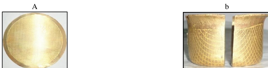
Fig. 6: A) grid square on the blank, B) Sample of forming grid cap
