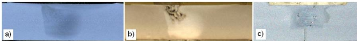
Fig. 5 – Examples of FS welds used to test the QNDT_FSW system
