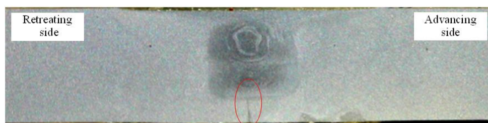
Fig. 8 – Macrograph of section 15 of the second application sample trials. Note the large root flaw due to incomplete penetration of the FSW tool
