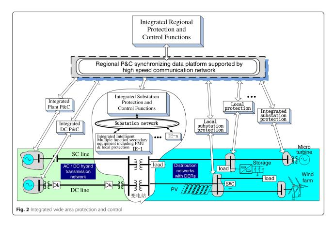
ensure reliability, together with other integrated functions such as fault recorder, data storage and network analysis, etc.
