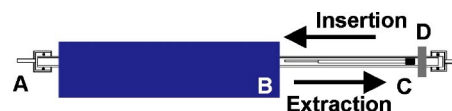
FIG. 1. (Color online) Schematic of: (A) 5.5 ft quartz tube (inner diameter: 22 mm o.d.; 25.8). Note endcaps and gaskets providing separate nonambient atmosphere. (B) Lindberg/Blue furnace box. (C) Rapid sample insertion and withdrawal apparatus. (D) Plastic coated ferrite ring magnet.
