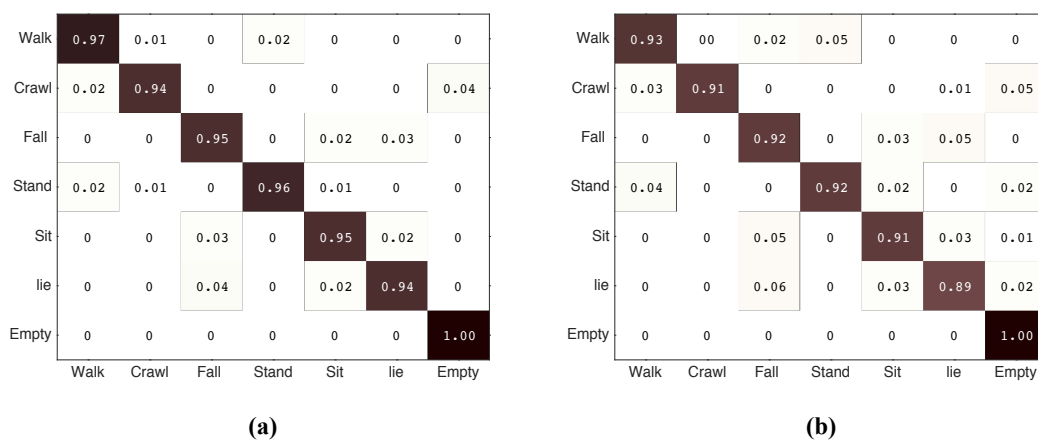
Figure 6. Confusion matrices for the activities classification. (a) confusion matrix for Line-of-Sight (LOS); and (b) confusion matrix for Non-Line-of-Sight (NLOS).
