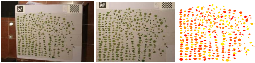
(a) Image of leaves placed on a table, captured through a DSLR camera. (b) Unwarped image after a perspective calibration board placed in the right top corner of the table. (c) Individual leaves detected using an image segmentation algorithm, leading to the computation of individual and total leaf area.
