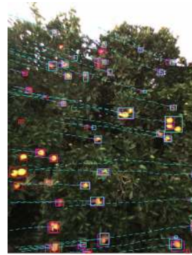
(b) Red boxes show detection of fruits, and cyan boxes show new fruits that were counted in the frame. Cyan lines show the paths of detected fruits from previous frames into the current frame. The purple boxes show predicted positions of the fruits detected in previous frames.
