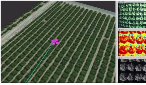
Fig. 9: ROS Rviz screenshot showing the UAV in flight above a row of orange trees in Booth Ranches, CA. The panels on the right show RGB, NDVI, and IR images acquired by the IRIS sensor suite onboard the UAV (top to bottom). NDVI imagery is generated using data from the multi-spectral cameras of the sensor suite.
