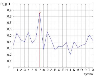
Fig. 12. Plot of the cross-correlation function for the symbols in a license plate; a maximum corresponds to symbol "7"
