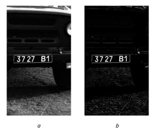
Fig. 4. Results of preliminary processing of the original image (Fig. 3): a – the result of the pixel-to-pixel multiplication of channels in the RGB color space; b – the result of using the morphological operation imtophat
