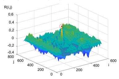
Fig. 6. An example of the surface of the cross-correlation function for the image of a vehicle's license plate (Fig. 4, *b*) and the sample (Fig. 5, *b*)
