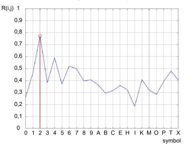
Fig. 13. Plot of the cross-correlation function for the symbols in a license plate; a maximum corresponds to symbol "2"
