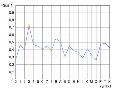
Fig. 11. Plot of the cross-correlation function for the symbols in a license plate; a maximum corresponds to symbol "3"
