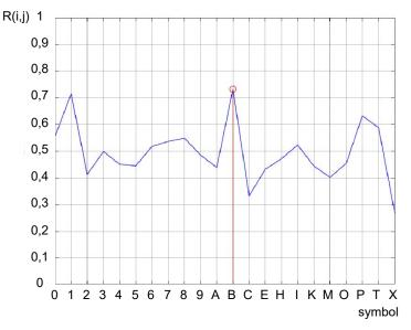
Fig. 15. Plot of the cross-correlation function for the symbols in a license plate; a maximum corresponds to symbol "B"
