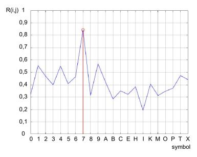
Fig. 14. Plot of the cross-correlation function for the symbols in a license plate; a maximum corresponds to symbol "7"
