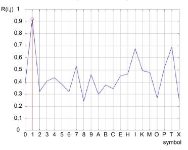
Fig. 16. Plot of the cross-correlation function for the symbols in a license plate; a maximum corresponds to symbol "1"
