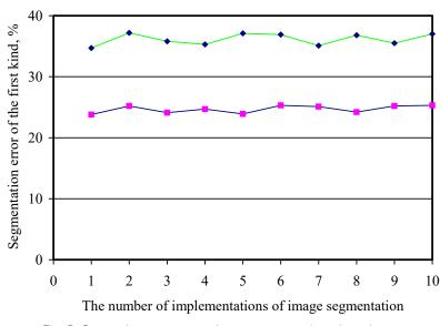
Fig. 5. Calculating a segmentation error of the first kind with the implementation of image segmentation from 1 to 10
