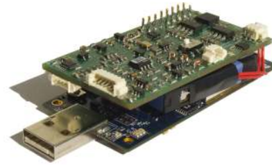
Figure 4. Illustration of the physiological sensor board (top) connected to the TelosB network node (bottom). The middle layer is a Li-ion battery.
