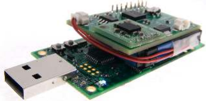
Figure 3. Illustration of the motion sensor node. The sensor board on the top is a custom-built motion sensor with a triaxial accelerometer and a biaxial gyroscope. The middle layer is a Li-ion battery. The sensor board on the bottom is a standard TelosB network node.
