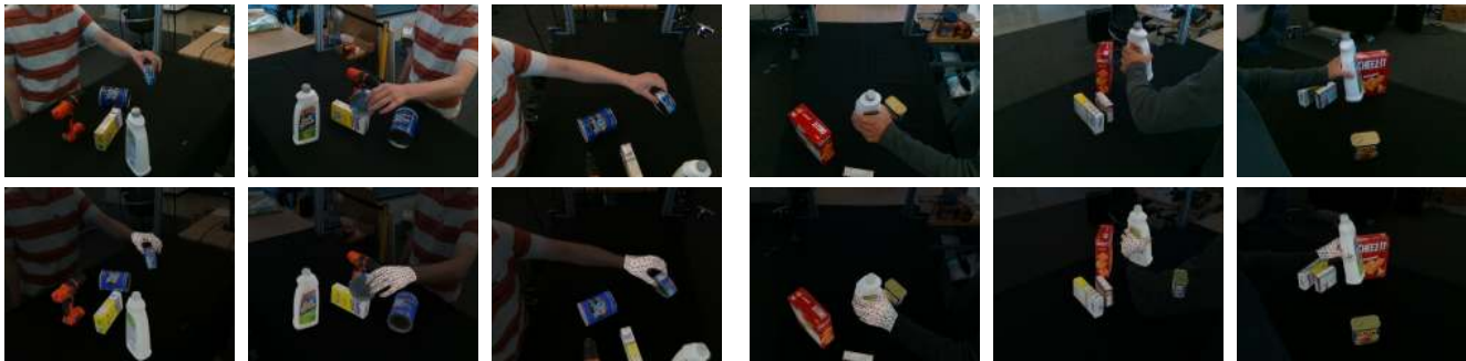
Figure 1: Two captures (left and right) from the DexYCB dataset. In each case, the top row shows color images simultaneously captured from three views, while the bottom row shows the ground-truth 3D object and hand pose rendered on the darkened captured images.
