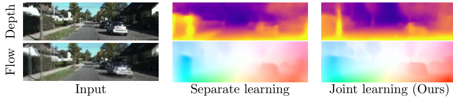
Fig. 1: Joint learning v.s. separate learning. Single-view depth prediction and optical flow estimation are two highly correlated tasks. Existing work, however, often addresses these two tasks in isolation. In this paper, we propose a novel cross-task consistency loss to couple the training of these two problems using unlabeled monocular videos. Through enforcing the underlying geometric constraints, we show substantially improved results for both tasks.
