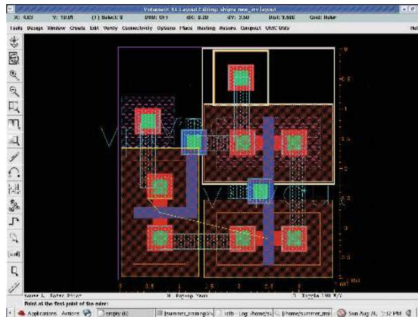
FIGURE 4: Layout of proposed DFAL inverter.
