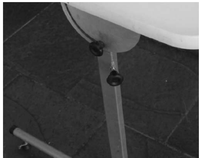
Figure 4. The clamping knobs of the table. Source: elaborated by the authors.
