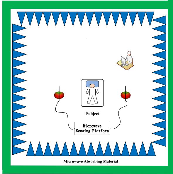
Figure 1–Experiment setup for detecting sleep apnea.
