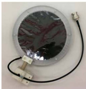
Figure 8. Picture of the SEM detector developed for the ELIMAIA beamline.
