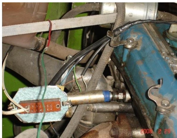
Fig. 12. Strain gauge pressure sensor connected to the central oil line by means of a connector and a signal amplifier integrated in one housing with the pressure sensor.
