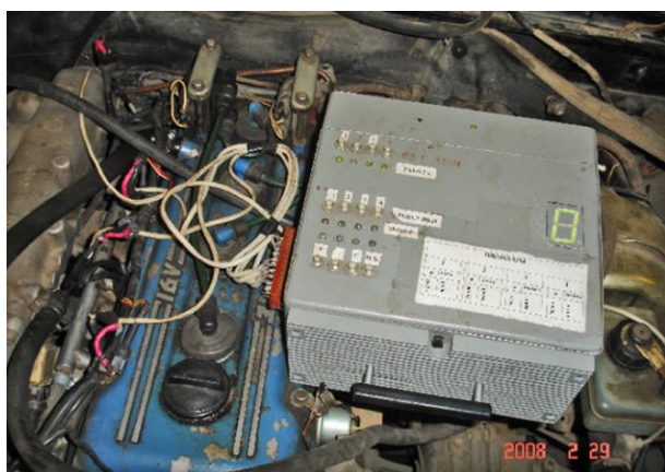
Fig. 10. Switch of electromagnetic injectors (engine loader) in the operating conditions when diagnosing the ZMZ-4062 engine.
