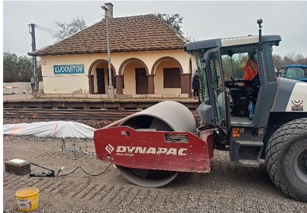
Fig. 5: Implementation of the static load test at the level of the sub-ballast upper surface in the area of the Ľudovítov stop and level crossing.
