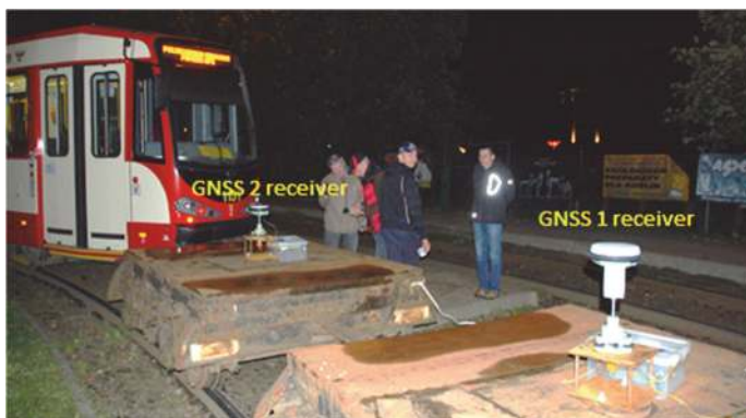
Fig. 1. Configuration of GPS/Glonass receivers on the platform
