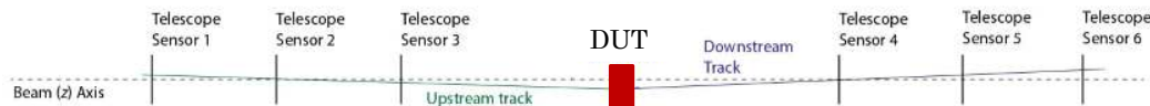
Fig. 11: Setup of the DATURA telescope. Tracks are independently reconstructed on each arm.
