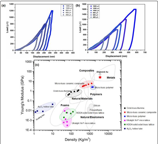
**Fig. 3 Nanoindentation tests for well-ordered nanonetwork Au.** The load-displacement curve of the well-ordered nanonetwork Au fabricated by using (a) Berkovich indenter and (b) spherical indenter under loads of 400 μN, 600 μN, 1000 μN and 1200 μN at a loading rate of 60 μN/s. **c** Comparison of Young's modulus versus density with different porous materials.
