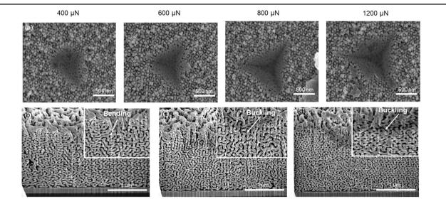
**Fig. 4 Microscopic analysis of post-indentation locations. a** FESEM micrographs of diamond-structured Au after nanoindentation using maximum loads of 400 μN, 800 μN, 800 μN, and 1200 μN with the use of Berkovich indenter. Cross-sectional-view SEM of diamond-structured Au after nanoindentation using spherical indenter with the maximum loads of (**b**) 400 μN (**c**) 800 μN and (**d**) 1600 μN.
