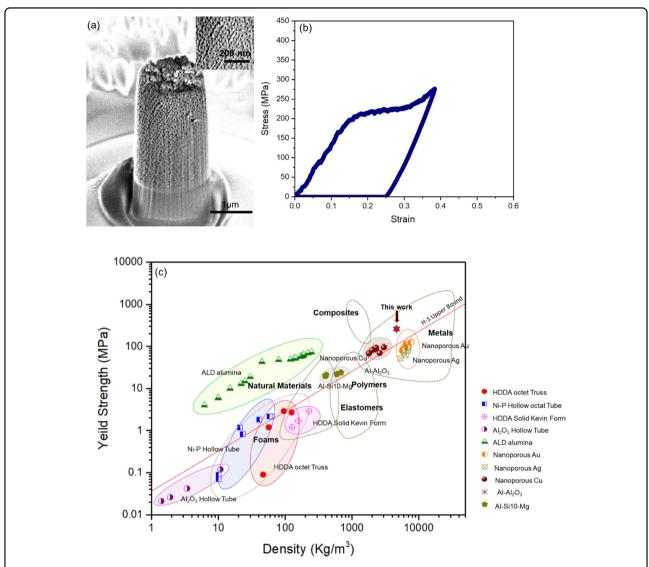
**Fig. 5 Mechanical characterization of diamond-structured Au. a** FESEM image of diamond-structured Au micropillar before uniaxial microcompression. The inset shows the enlarged image of the sidewall of the micropillar. **b** Engineering stress-strain curves of diamond-structured Au. **c** Yield strength vs density material property chart comparing different porous metals with nanonetwork Au.
