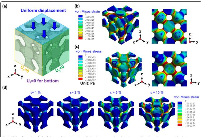
Fig. 6 Finite element analysis of diamond structured Au. a Finite element model and boundary condition b von Mises stresses distribution c von Mises strain distribution and d Equivalent strain at different strain levels  $\varepsilon = 1\%$ ,  $\varepsilon = 2\%$ ,  $\varepsilon = 5\%$ , and  $\varepsilon = 10\%$ .
