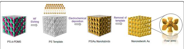
Fig. 1 Design and fabrication process. Schematic illustration for fabrication of well-ordered nanonetwork Au from a bottom-up approach.
