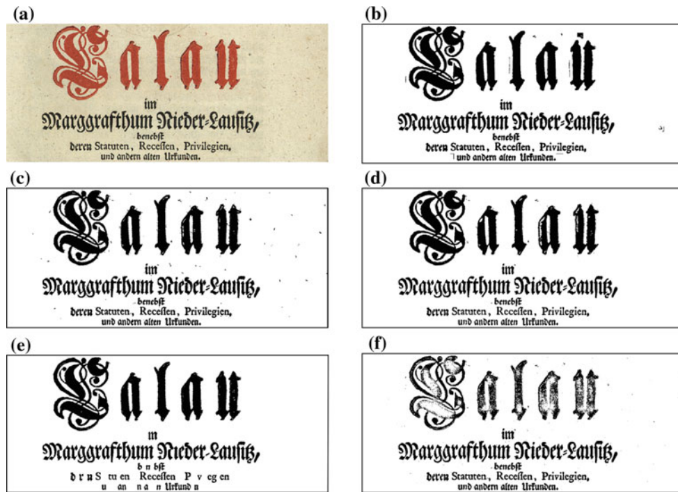
Fig. 1 a Representative machine-printed image; b–f Binarization results from the first to the fifth best binarization algorithm, i.e. algorithms No. 26, 14, 24, 10 and 9a, respectively
