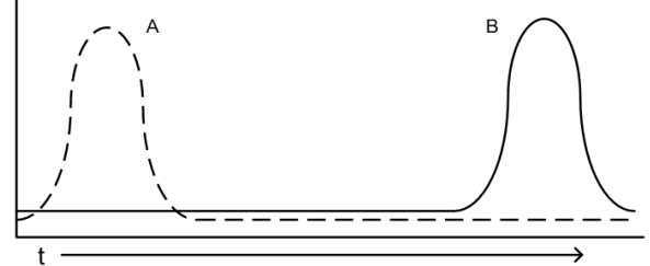
Fig. 4. The \delta factor is used to control dictionary segments from being improperly used. Here, segments that are produced by the peak of time-series A could be used during the compression of the peak of target series B. Further, both time-series have flat intermediary regions that are within small \epsilon . The compression sizes would be quite similar and erroneously give favorable similarity.
