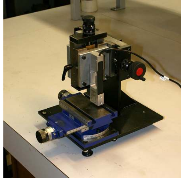
Figure 6: The shear tester used (specific development), with a 20 kgf (200 N) load cell mounted
