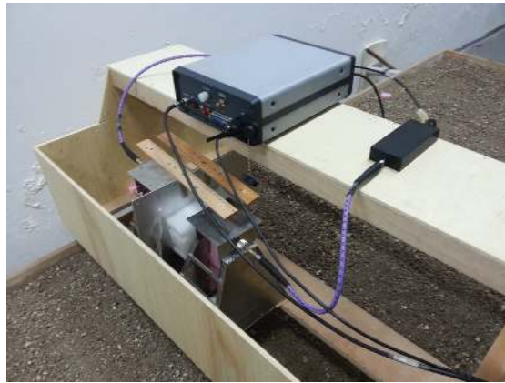
Figure 9. Test and measurement setup of 15 GHz impulse GPR system.
