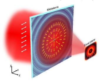
**Figure 1.** Schematic illustration of the superoscillatory focusing metalens. The arrows depict the instantaneous directions of electric component of the light field input and output from the metalens.
