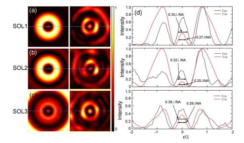
**Figure 5.** Experimental results of three superoscillatory metalenses. (**a**–**c**) Intensity distributions of the simulated and measured focal fields generated by metalenses with parameters of  $k_r = 0.08k_0$ ,  $0.29k_0$ , and  $0.43k_0$ ; (**d**) Normalized line-scan intensity profiles at the focal plane (indicated by dashed lines): simulation (red) and experiment (black).
