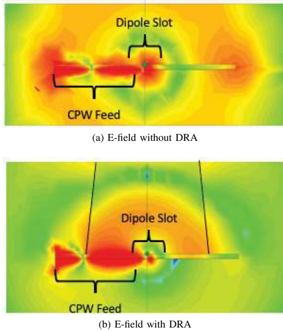
Fig. 6: Comparison of the electric field in the CPW feed and folded dipole slot with and without the DRA viewed normal to the CPW feed, along the folded dipole slot. The dipole pattern is seen in a). The beginning of the formation of the surface wave is seen in b).
