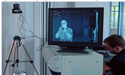
Fig. 1.3 Thermal imaging camera to detect fever, one of the signs of infection
