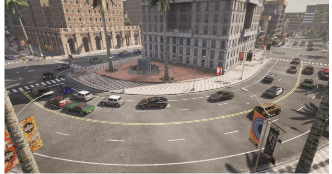
Fig. 1. Traffic simulation in an urban environment. Traffic simulation can be used to analyze complex traffic dynamics. Among two popular traffic models, by simulating areas of interest with the microscopic one and using macroscopic simulation elsewhere, we can reduce the overall computational cost without compromising significant details. For instance, the center of intersection can be simulated with discrete, agent-based models for higher-fidelity inter-vehicle dynamic interaction. ( This scene is rendered in CARLA [Dosovitskiy et al. 2017]. )
