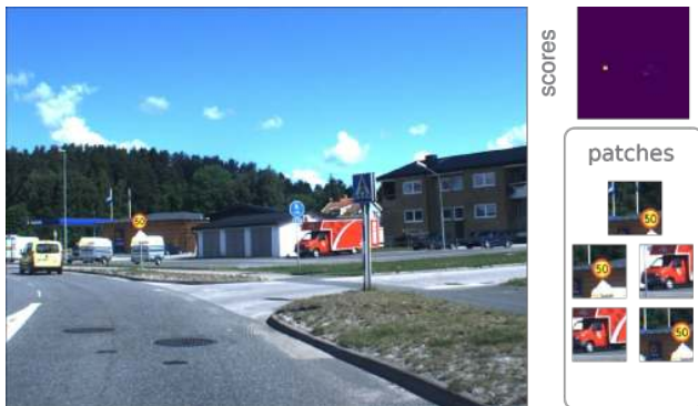
Figure 5: Left : Example of a 960 \times 1280 image from the traffic signs dataset. Top-right : scores predicted for patch extraction. Right : Patches extracted by perturbed Top-K at inference.
