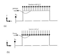
Figure 1: Axial section of the channel in case of (a) suction (b) injection
