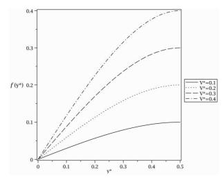
Figure 3: Effects of the injection velocity  $(V_0)$  for  $f(y^*)$  on the 15th-order approximation (M = 1, Re = 4)
