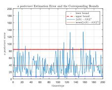
Fig. 2: The squared error of the cloud's state estimates (solid line), the lower bound on estimation error in Theorem 1 (dotted line), and the upper bound on estimation error in Theorem 1 (dashed line) over 200 timesteps. We see that instantaneous a posteriori error typically obeys our MSE bounds, and on average lies within the bounds.
