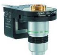
High-speed nanofocus <1nm resolution
