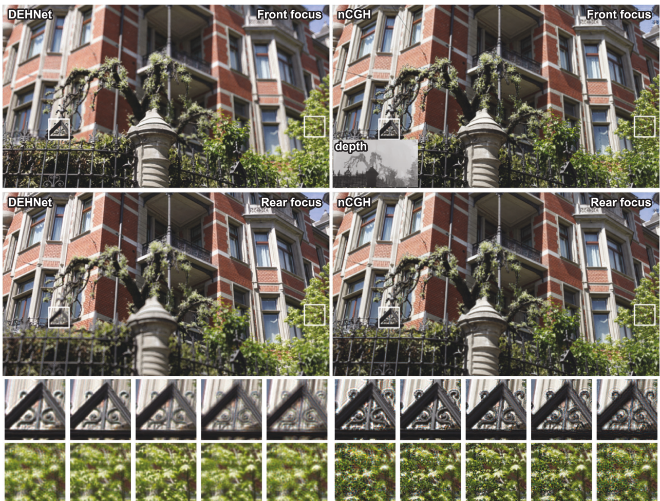
Fig. 6 | Simulation results obtained using a real-world RGB-D image. Using a real-world-captured image 39 , a DEH and an nCGH were synthesized and their intensities were simulated wherein the total image size was resized to 1280 \times 720 . The large images show the front- and rear-focused images, while the small images
