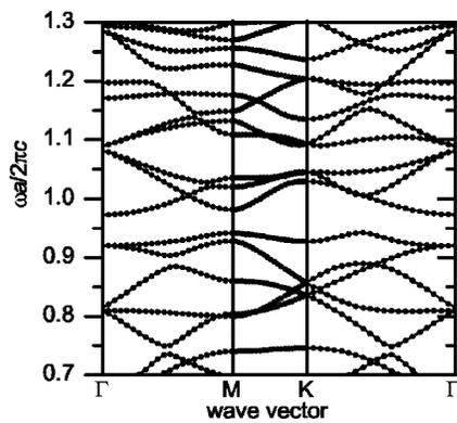
FIG. 2. Band structure of the higher-order bands for the photonic crystals investigated ( $r/a=0.4$ ,  $H$  polarization). The fundamental band gap can be found around  $\omega a/2\pi c_0=0.3$  and is not investigated in our experiments.
