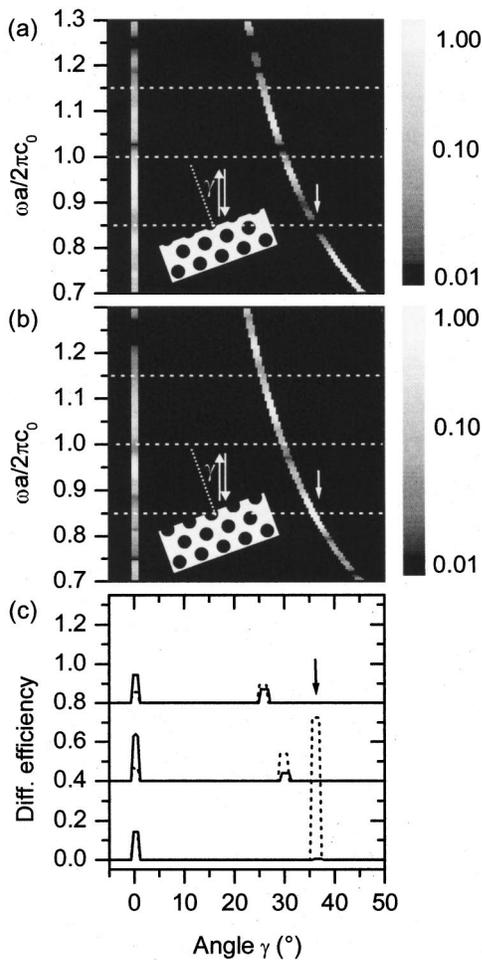
FIG. 4. (a) Complete numerical simulation for a 2D-PC cut along the  $\Gamma M$  direction. (b) Same as (a) but for a different surface termination as indicated by the insets. The arrows mark the same position as in the experiment [see Fig. 3(a)]. (c) Cuts at the same positions as in the experiment. The solid curves correspond to (a), the dotted ones to (b).
