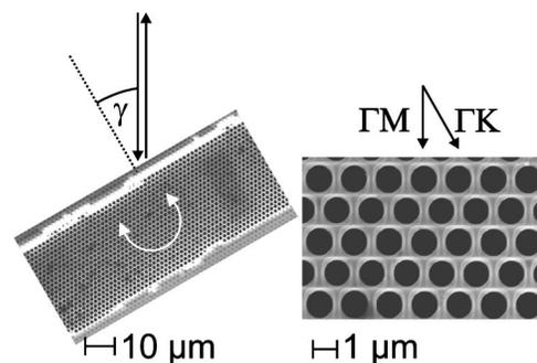
FIG. 1. One of the photonic crystals investigated, cut along the  $\Gamma\text{K}$  direction. The angle of incidence  $\gamma$  with respect to the normal coincide with the detection angle. The magnification shows the high quality of the internal structure. The  $\Gamma\text{M}$  and  $\Gamma\text{K}$  directions are emphasized.
