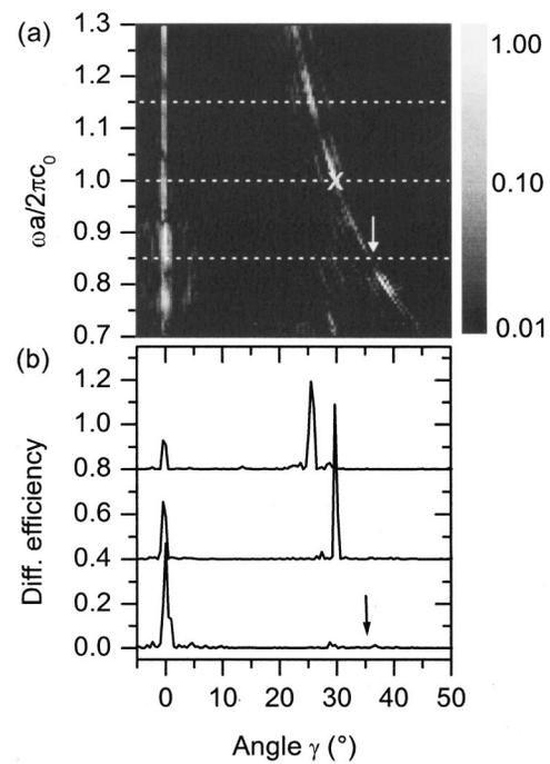
FIG. 3. (a) Measured intensity diffraction efficiency for a cut along the  $\Gamma K$  direction. The arrow marks a region of diffraction efficiency  $< 5 \times 10^{-3}$ . The cross marks the position of the Bragg reflex expected for an ideal 2D structure. (b) Cuts at selected spectral positions, as marked by the dotted lines in (a). The spectra are vertically offset for clarity.
