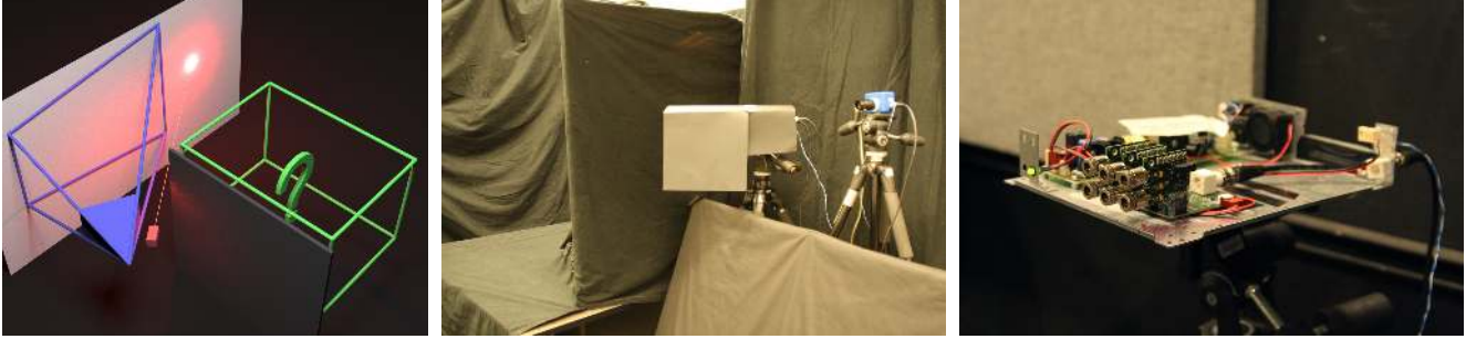
Figure 2. Left: 3D model of our setup (to scale). Center: Photo of our capture setup facing the diffuse wall (light source covered with black photo board). To the left, behind an occluder, lies the reconstruction volume. Right: Close-up on the light source without cover.
