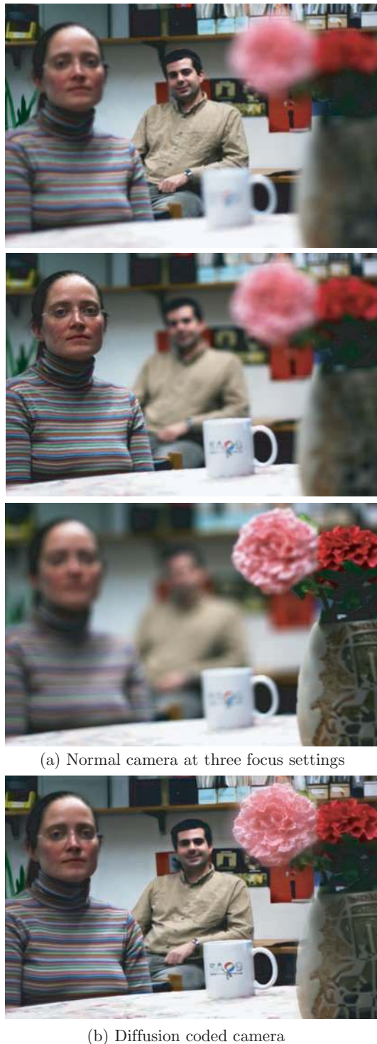
Figure 14: Extending DOF with diffusion coding. All images were taken with a 16ms exposure time. (a) The top, middle, and bottom images were captured using a 50mm f/1.8 Canon lens focused on the background, middle, and foreground, respectively. The depth of field is too narrow for all objects to be in focus simultaneously. (b) The diffuser from Section 6 is inserted into the lens aperture and deblurring is applied to recover the EDOD image in (b). Diffusion coding results in a roughly 10\times increase in DOF.
