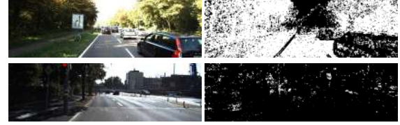
Figure 5. Auto-masking. We show auto-masks computed after one epoch, where black pixels are removed from the loss ( i.e. \mu = 0 ). The mask prevents objects moving at similar speeds to the camera (top) and whole frames where the camera is static (bottom) from contaminating the loss. The mask is computed from the input frames and network predictions using Eqn. 5.
