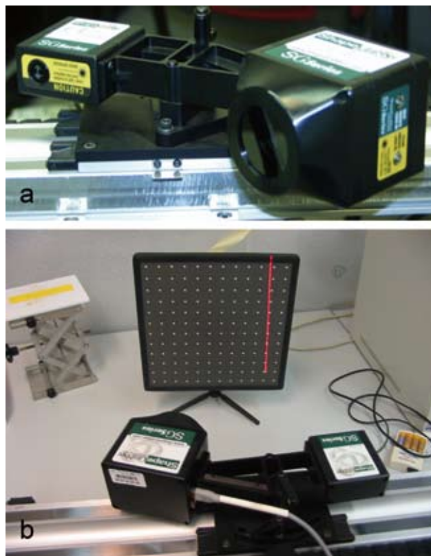
Fig. 8 - a. ShapeGrabber SG1002 head; b. ShapeGrabber SG1002 calibration procedure.
