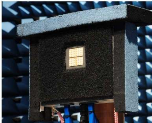
Figure 6: 8x8 Rx array mounted on the manifold in an anechoic chamber.
