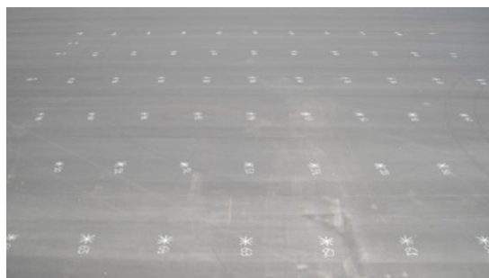
Figure 4. Field calibration surface with the targets points
