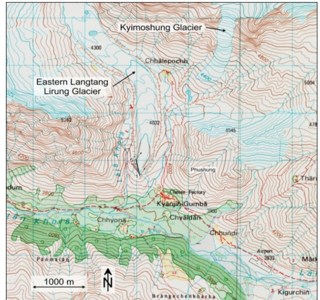
Figure 6. Clip of the topographical map 1:50,000 (sheet number 2885 15) showing the study area with Kyimoshung Glacier and Kyanjin Gumpa. Compare with Figure 2. The photogrammetric baseline (1-5) for mapping Kyimoshung Glacier was added graphically. Map © Survey Department, Kathmandu, Nepal
