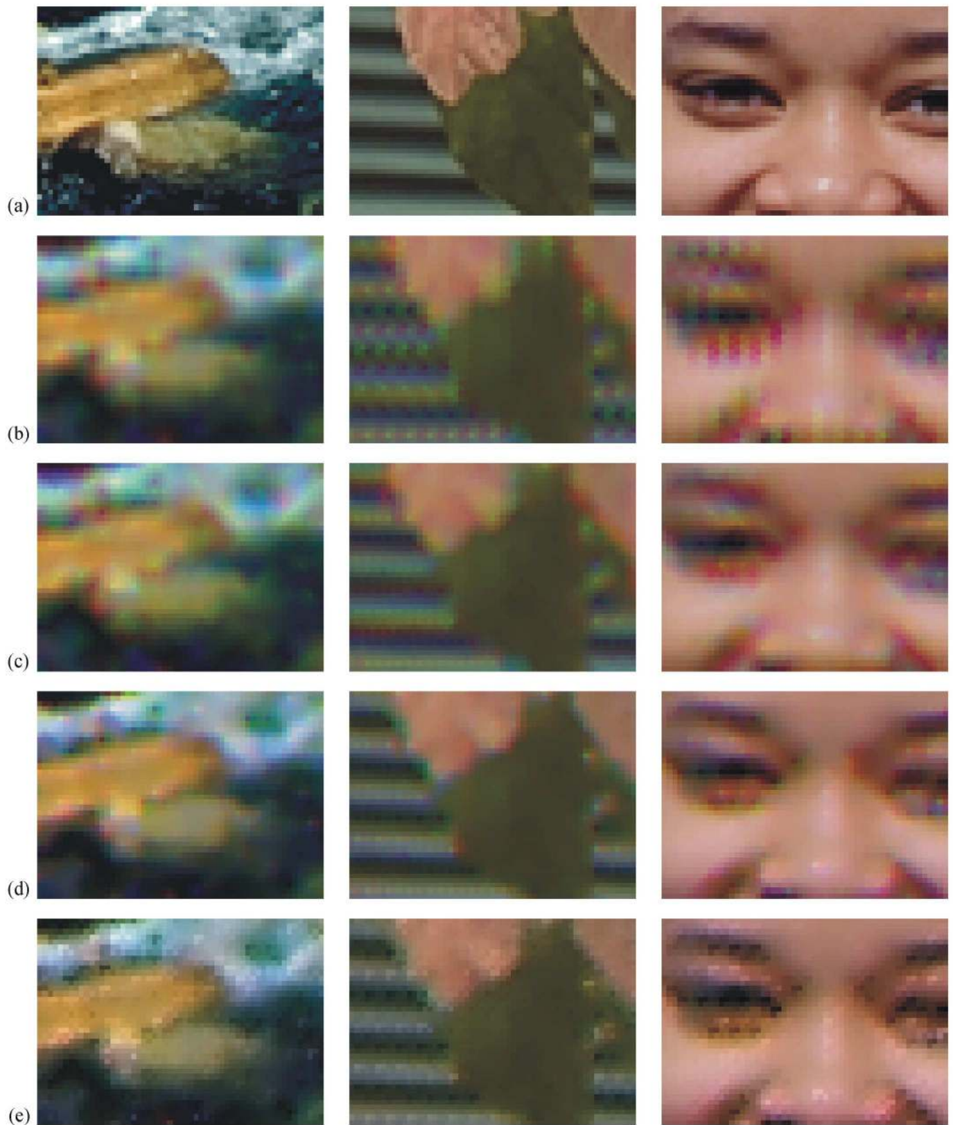
Fig. 8. The selected portion of the results achieved using the test image Mountains (left column), Window (middle column) and Girls (right column) and the following method: (a) original image, (b) CIZ scheme, (c) LZ scheme, (d) CDES scheme, (e) proposed unified scheme.
